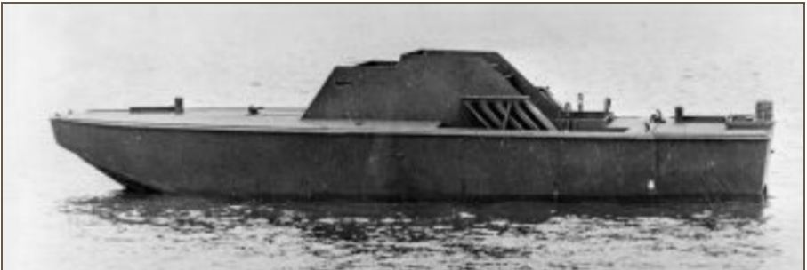
20 An LCS(S) rocket boat, LCS(S)-2, off New Orleans in 1944. Two joined the Calvert on 1 April 1943, each with a crew of five, machine guns and 96 bombardment and 42 smoke rockets. Naval Institute Archive.
